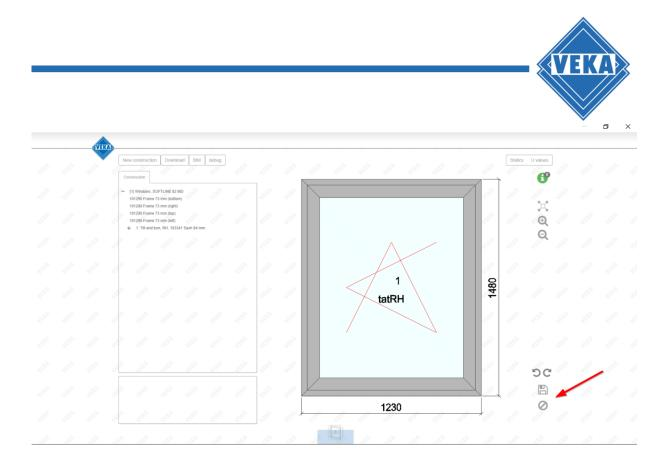
The construction data are now transferred to Revit<sup>®</sup> and, depending on the design, a window or door Family File (.rfa) is created, saved and opened.
