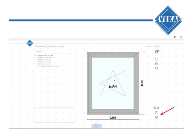
The construction data are now transferred to Revit<sup>®</sup> and, depending on the design, a new family window or door is created, loaded into the project and selected directly. The newly created window or door can now be inserted into a wall.
